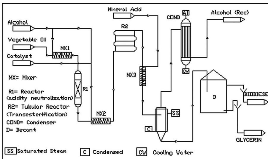
Fig. 1 – Biodiesel fuel production scheme. Adapted from [2].
