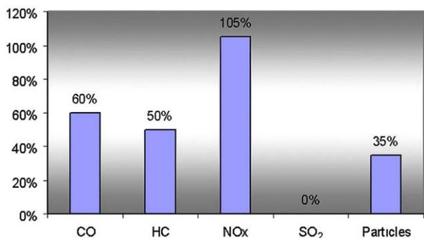
Fig. 2 – Gaseous emissions of biodiesel combustion in an internal combustion engine. The value of 100% is considered the emission level of the diesel engine [7].
