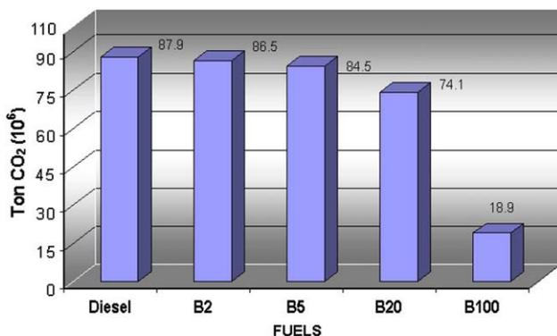
Fig. 7 – CO<sub>2</sub> emissions by fuel type, for the last five years, for the Brazilian diesel fleet.
